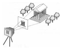
For convenience, the image plane is usually placed in front of the camera, giving a non-inverted 2D projection (image).
