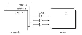
The term **true-color** is sometimes used to refer to systems which the framebuffer directly stores the values of each channel.
