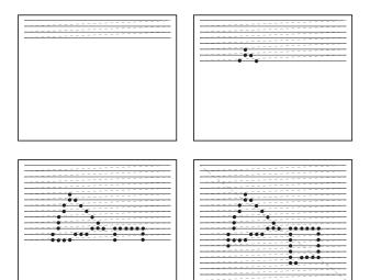
Electron beam traces over screen in **raster scan** order.
